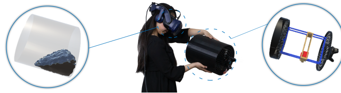
Figure 1. SWISH, a haptic feedback device capable of simulating fluid behavior in virtual reality or augmented reality. (Left) simulated virtual fluid in virtual reality, (Right) the mechanically actuated system that tangibly represents a fluid's center of gravity.
