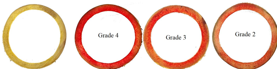
Fig. 3 Boron penetration analysis of samples treated with DOT (untreated reference sample at left). Grade 4 (>75% penetration); Grade 3 (50–75% penetration); Grade 2 (25–50% penetration)
