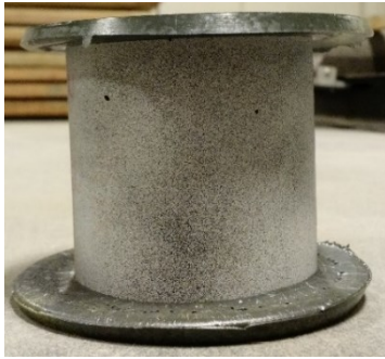
a) compression specimen showing sulphur capping and DIC speckle pattern. Specimen height is approximately 90 mm.
