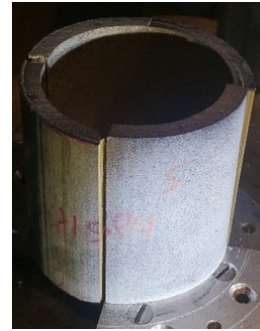
b) "bowtie" test set-up and typical specimen failure. Specimen height is approximately 90 mm.
