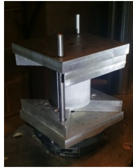
b) "bowtie" test set-up and typical specimen failure. Specimen height is approximately 90 mm.
