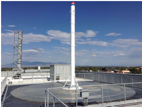
Figure 2. Solar chimney power plant model on the roof of the Aerospace and Mechanical Engineering building at the University of Arizona.
