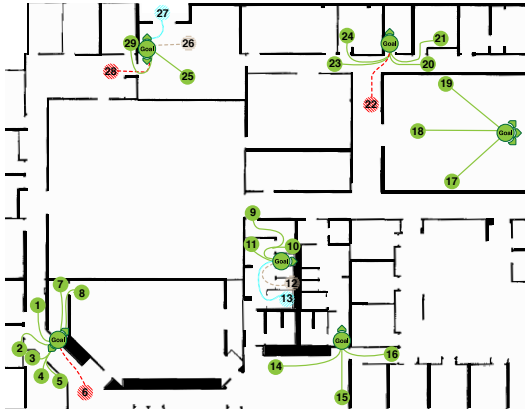
Fig. 5: The 29 trajectories we evaluated. The green arrows next to goal poses show desired ending orientations. Green trajectories were completed by both planners, red trajectories were only completed by RobotOnlyPlanner, blue trajectories were only completed by CoupledPlanner, and grey trajectories were completed by neither.
