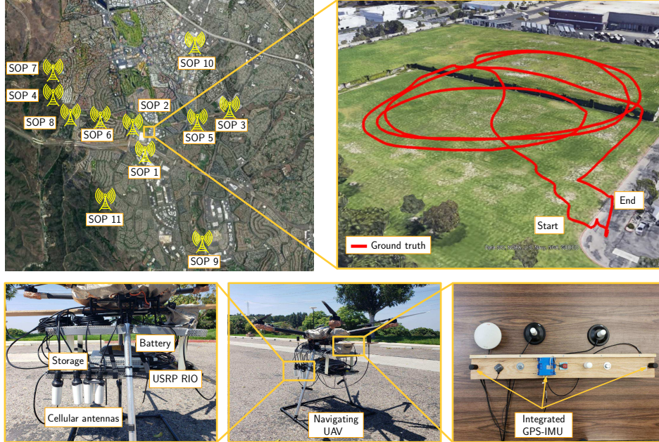
Fig. 5. Experimental hardware setup and the traversed trajectory along with the position of cellular LTE SOP towers. A UAV was equipped with an integrated AsteRx-i V GNSS-IMU system, cellular antennas, and a USRP. The UAV traveled 823 m in an urban area (Irvine, California, USA) collecting GPS and cellular LTE signals from 11 cellular LTE SOP towers.
