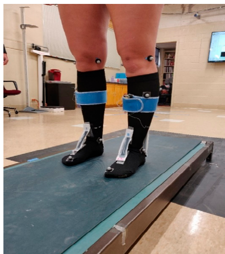
Figure 1. Arrangement of SRS and motion capture marker setup to capture and assess sagittal plane ankle kinematics (PF and DF), positioned on a treadmill belt to provide external postural perturbation in the forward and backward direction. SRS: soft robotic sensor. PF: plantarflexion. DF: dorsiflexion.
