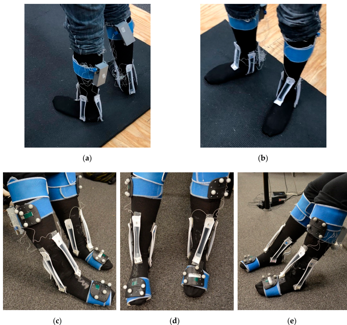
Figure 2. Soft robotic sensor placement and orientation configuration or SRS POC placement for the (a) left and (b) back for a simulated participant at rest prior to a TSP gait trial; SRS POC placement and motion capture marker set placement for the (c) left, (d) front, and (e) right for stimulated seated participant.
