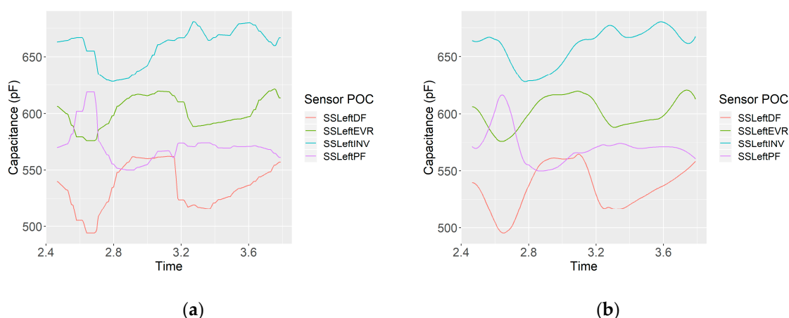
Figure 6. (a) Upsampled StretchSense™ gait cycle data for the left foot collected before filtering. (b) Upsampled StretchSense™ gait cycle data for the left foot after filtering (third-order, window length of 39).
