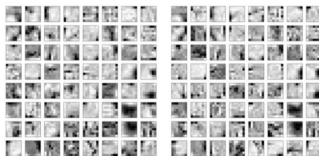
FIGURE 5 | 7 \times 7 Filters learned in the positive polarity channel (Left) and negative polarity channel (Right) of the first convolutional layer. The similarity of the kernels across the two polarities reflects the DVS data, where leading edges and trailing edges co-occur with opposite polarities.
