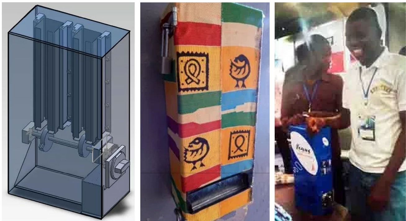
Fig. 4 The DIY condom-vending machine: open source blueprints, Adinkra skin, and blue paint final version
