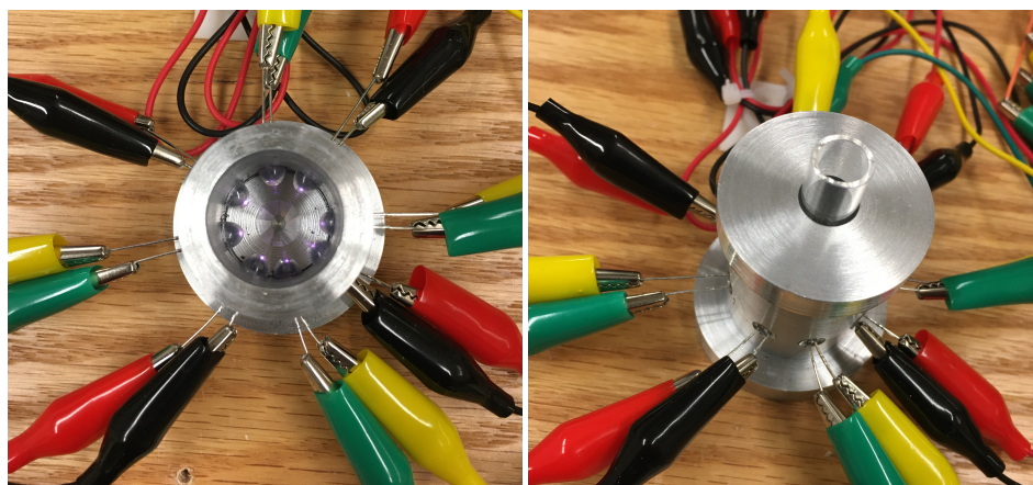
Figure S8. Photolysis apparatus equipped with eight 350 nm LEDs arranged in a radial manner. Left: Apparatus without top. Right: Apparatus with top showing reaction tube inserted into the center.
