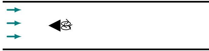
Fig. 1 The schematic of the bluff-body combustor geometry developed by the US Air Force Research Lab (AFRL).
