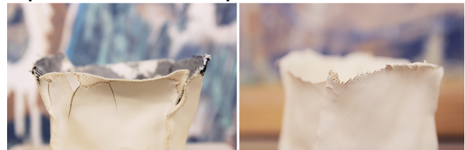
Figure 7. (Left) slip dried on the fabric scaffold. (Right) the flaky edge on the bisque resembles the texture of the fabric.
