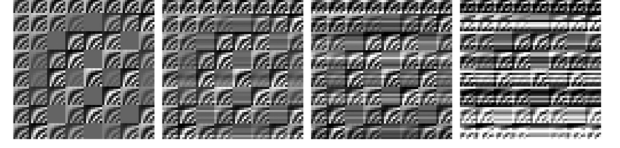
Fig. 1. Learning a dictionary from increasingly noisy data. The (unraveled) basis elements of the 8 \times 8 discrete cosine transform (DCT) form the 64 columns of the left-most matrix above. Three increasingly imprecise dictionaries (columns reordered to best match original) are recovered by FastICA [26] trained on data generated from 8-sparse linear combinations of DCT elements corrupted with additive noise (increasing from left to right).
