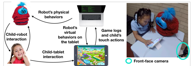
Figure 1: The integrated system for a robotic learning companion consists of a robot, a computer, a USB camera and a touch-screen tablet.
