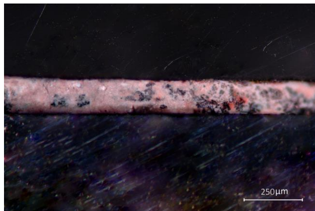
FIGURE 10: CROSS-SECTIONAL VIEW OF DEPOSITIONS USING 10X MAGNIFICATION OF LEICA DM2700
