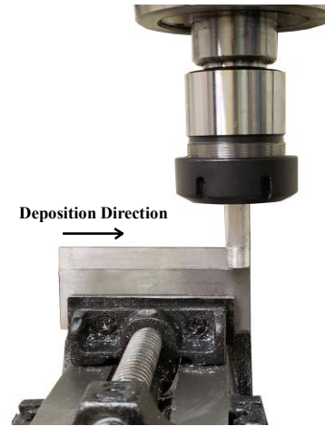
FIGURE 2: FRICTION SURFACING USING SIDE OF THE CONSUMABLE TOOL
