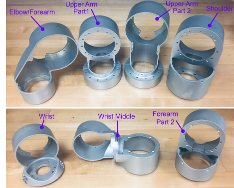
Fig. 10: Exoskeleton shell structural links. Each link is machined from a single block of 7075 aluminum using 5-axis milling.
