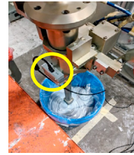
Figure 3: The box circled in red is the sensor box containing accelerometers mounted to the nozzle of the robot.
