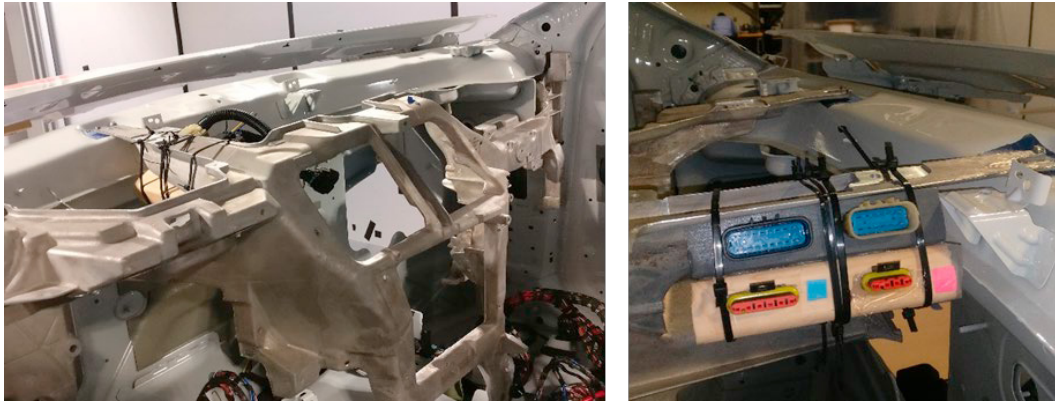
Fig. 6. (a) Metal plate with four screws for inspection (b) placement inside door cavity for obstructed assembly
