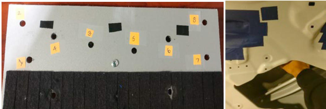
Fig. 5. (a) Metal plate with four screws for inspection (b) placement inside door cavity for obstructed assembly
