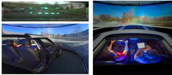
Figure 1: Lab's AR HUD can be display graphics that are both screen-relative and conformal to the simulated world (top left). Top view (right) and side view (bottom right) of driving simulator
