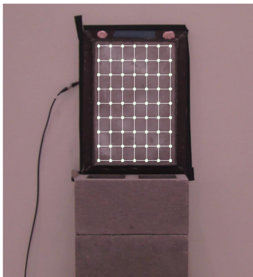
Fig. 4. (a) 7 \times 13 grid of scan points used to measure the surface velocities of the second panel. (b) Structural response of the second panel as measured by the SLDV.
