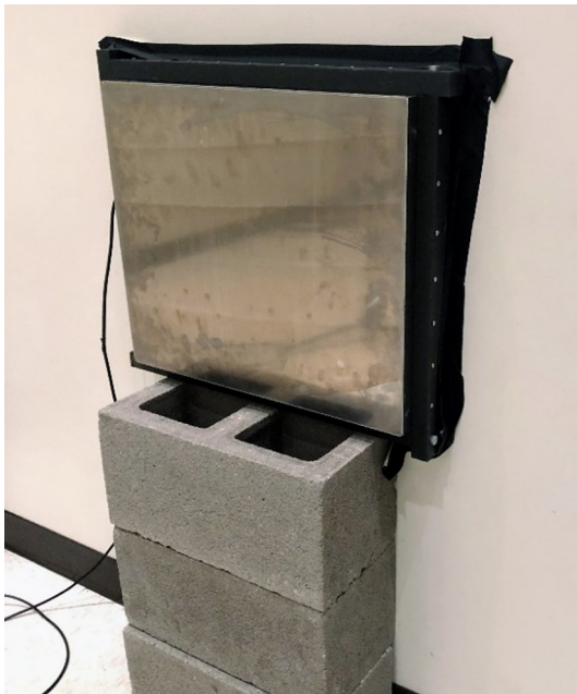
Fig. 1. Setup of a single panel in a reverberation chamber with the wall of the reverberation chamber acting as a baffle.
