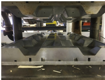
Fig. 19. New mold to fabricate the redesigned geometry.
