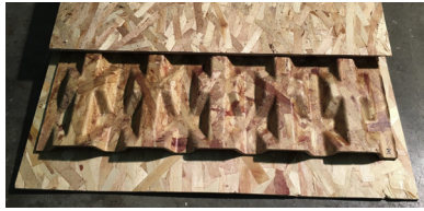
Fig. 1. Wood composite sandwich panel configuration; biaxial corrugated ore and flat panels.
