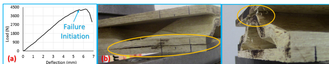
Figure 9. Four-point bending test of the sandwich specimens in the longitudinal direction: (a) typical load–deflection curve, (b) failure mode, delamination due to interfacial shear between the outer plies and the core.
