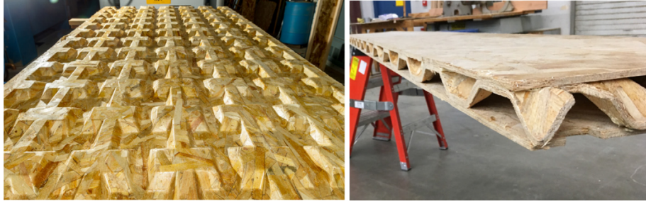
Fig. 1. Biaxial corrugated wood composite core and corresponding sandwich panel.
