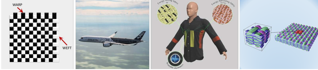
Figure 1: Woven Fabric in Engineering: Left to right—A schematic diagram of regular planar woven fabric; The Airbus A350-900 constructed by more than 50% composite materials [9]; A scheme of self-charging E-textiles by Pu et al. [10]; A schematic diagram of 3D woven fabric by Drach et al. [11]
