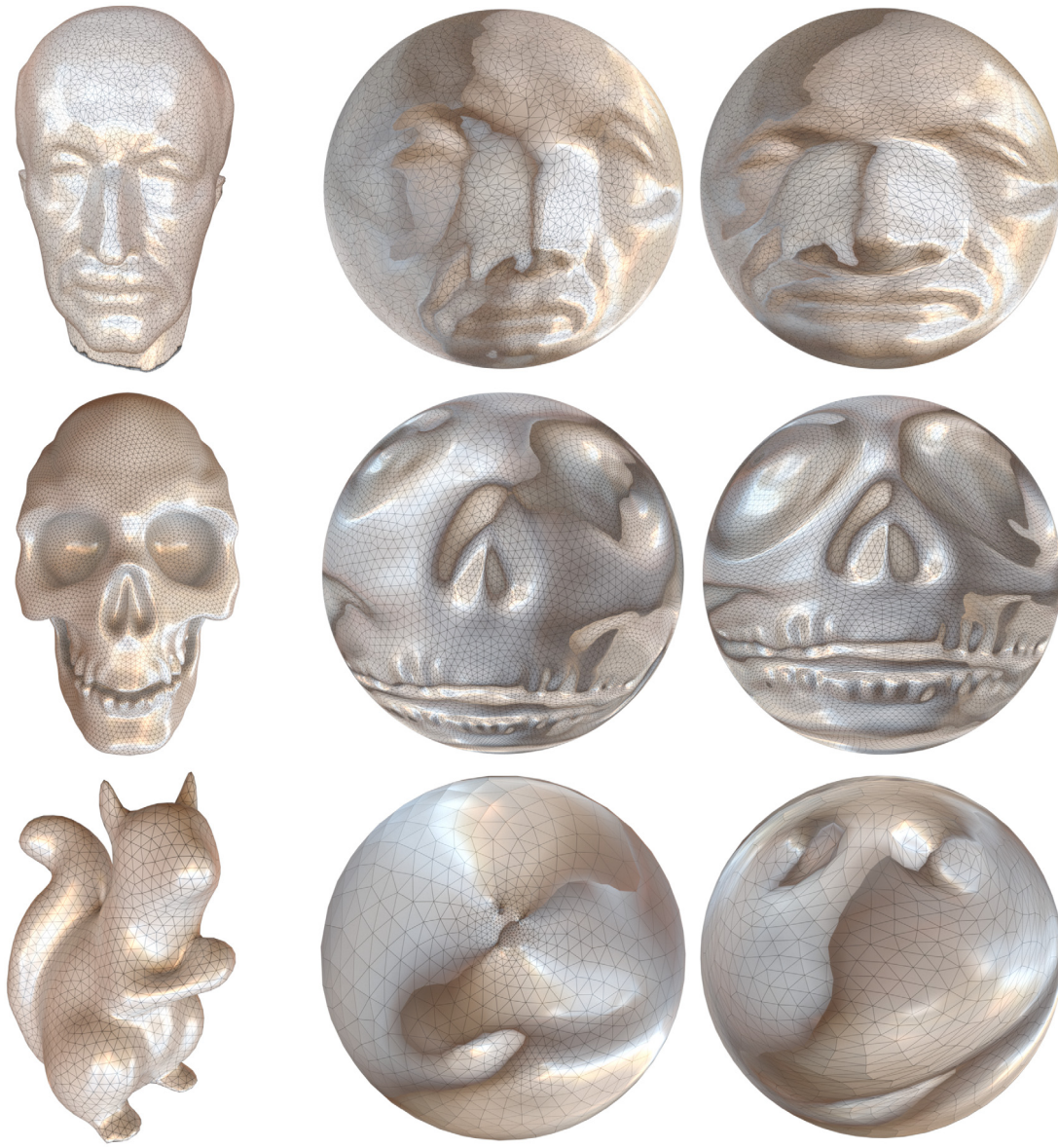
Fig. 14. Numerical experiments. Top row shows the Maxplanck model, and skull and squirrel models are shown in the middle and bottom rows. The original input surface, conformal mapping results and area-preserving mapping results are shown in left, center and right column accordingly.
