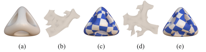
Figure 16: Image (a) is the original mesh cutted; (b and c) are the injective mapping and its texturing; (d and e) are the bijective mapping and its texturing.
