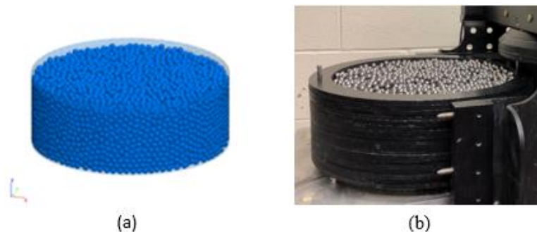
Figure 1 - (a) Numerical and (b) Experimental specimen of 10,636 chrome steel spheres
