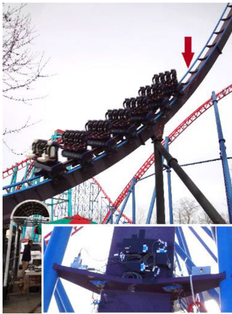
Fig. 5 Instrumented bracket location with close-up view of bracket and instrumentation
