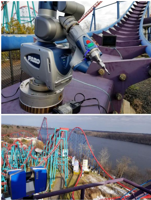
Fig. 10 Scanning of rollercoaster section. Top: 3D LiDAR Scanner. Bottom: CMM arm
