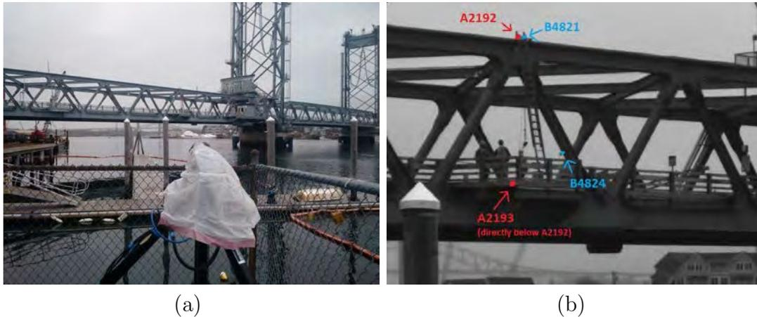
**FIG. 4. (a) Picture of the view from the camera with (b) screenshot from the recorded video with comments as to the locations of the accelerometers and strain gauges on the bridge. For A2192 the camera region of interest is centered on the accelerometer location as annotated with size  $218 \times 92$  pixels, while for A2193, the region of interest is directly below the A2193 sensor as annotated with size  $300 \times 76$  pixels.**
