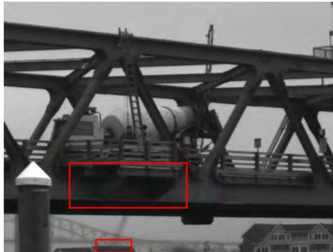
**FIG. 9. Screenshot from the start of the 10:21:03 am video showing a concrete mixer truck and regions of interest boxed on the bottom chord and an object in the background for reference**
