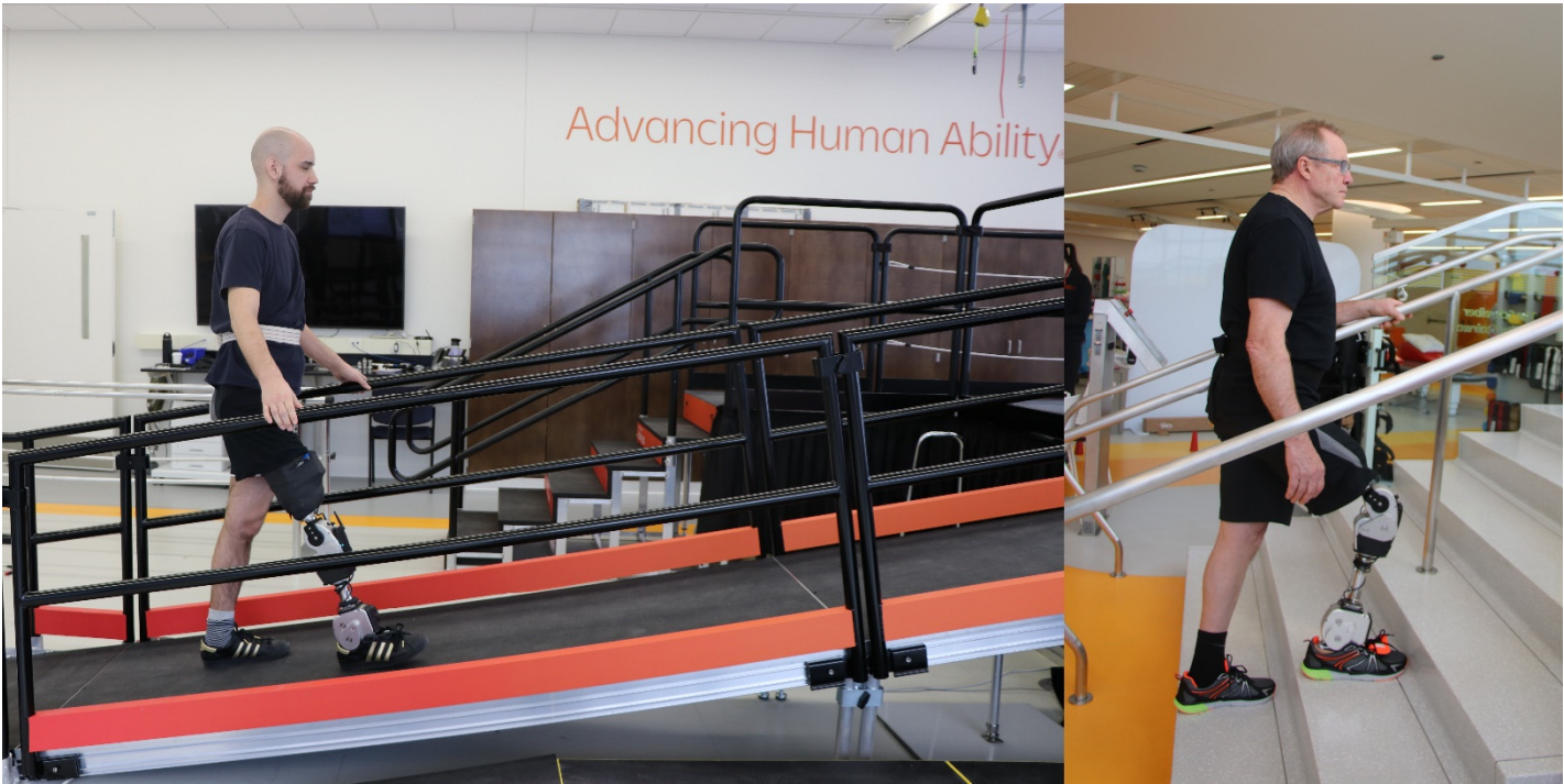
Figure 4 | Subjects with a transfemoral amputation ambulating with the OSL.
