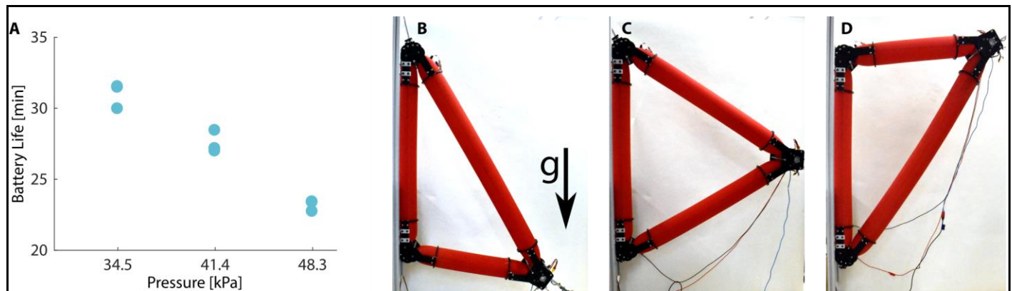
Fig. S1. (A) The battery life of a single roller module running continuously at three different pressures. We repeated the test three times per pressure. (B to D) The roller module is moved in a cyclic path. The roller module is a part of a triangle oriented vertically so that the roller module moves against gravity. The battery life calculated in (A) is extrapolated from the energy drawn and time elapsed during one cycle starting at a low point (B) moving upward to a high point (D) and then returning to the low point (B). The battery used for this calculation is a 14.8 V, 1300 mAh, LiPo battery.
