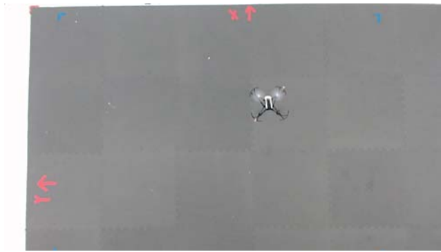
Fig. 2. For system identification purposes, the UAS was flown in a squared trajectory, at 1m above the floor (i.e., the X-Y plane) of the lab flight arena. A Motion Capture System and a ground control station were used for collecting input-output information for the UAS motions in the X and Y directions, at a rate of 100Hz.
