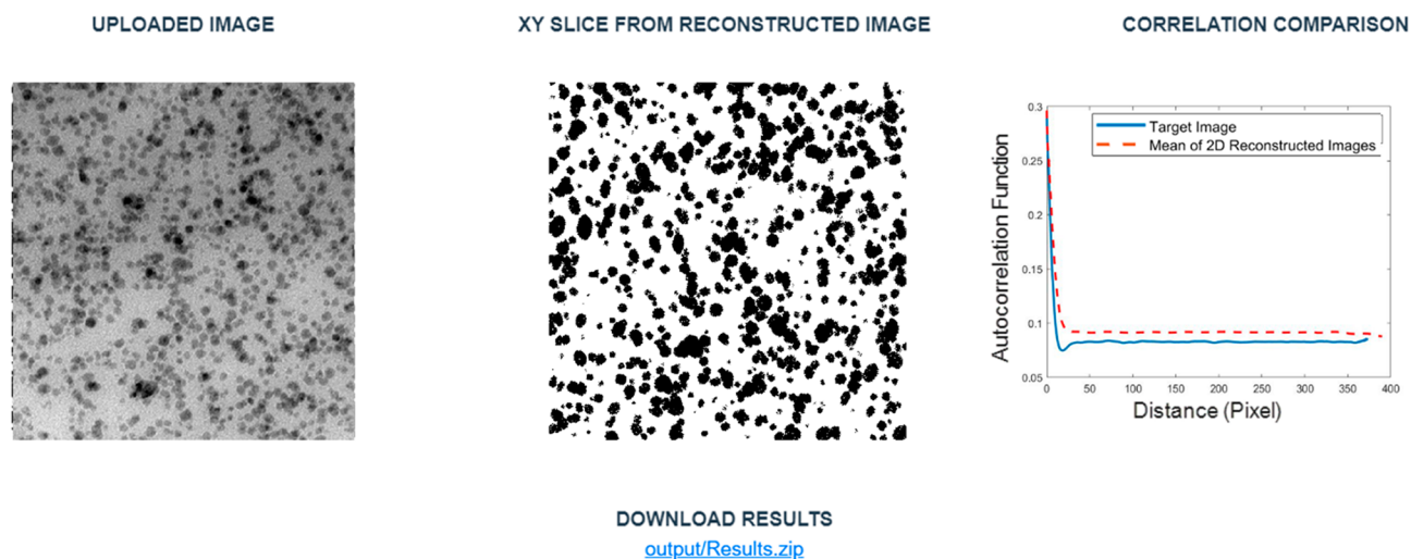
Figure 6. TEM image reconstruction using NanoMine. (Left) TEM micrograph of silica in poly(ethylene oxide) from Jimenez et al., 22 Copyright 2019 American Chemical Society. (Middle) One 2D slice from the 3D reconstruction of the original image using Physical Descriptor technique. (Right) Comparison of two-point correlation functions between reconstructed and original (target) images.
