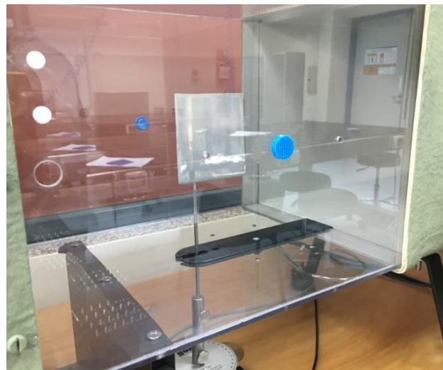
Figure 10: View of Educational Wind Tunnel HM 170 and designed experiment for wind tunnel testing.
