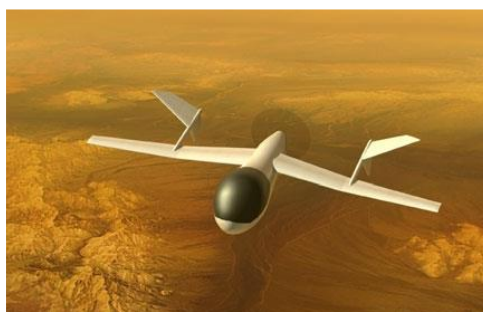
Figure 3. Schematic view of Aerial Vehicle for In-situ and Airborn Titan Reconnaissance (AVIATR) 19 .
