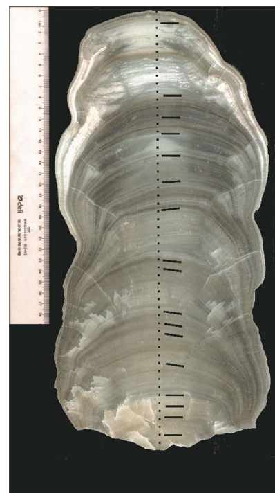
Fig. 2 Polished section of XL15. Black bars indicate positions of U-Th dates. Black dashed line shows the drilling path for the analysis of stable isotopes
