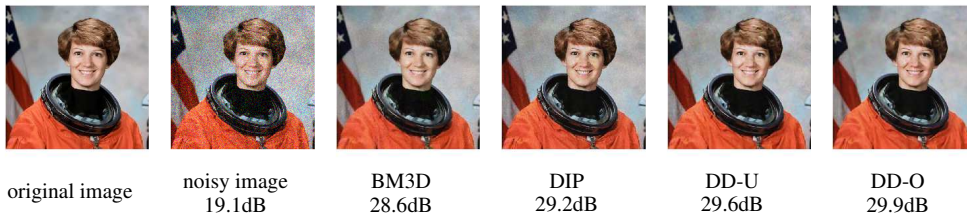
Figure 2: Denoising with BM3D and various convolutional generators. The relative ranking of algorithms in this picture is representative and maintained on a larger set of test images (see Appendix A). DD-U is an under-parameterized deep decoder. DIP and DD-O are over-parameterized convolutional generators and with early stopping outperform the BM3D algorithm, the next best method that does not require training data.
