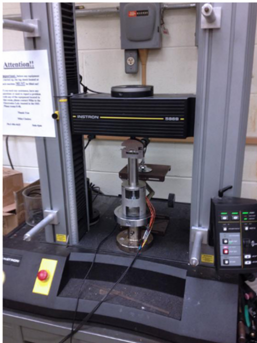
(b) Tensile test machine - Instron 5869
