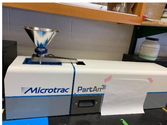
Fig. 3. A 3D particle size and shape analyzer.
