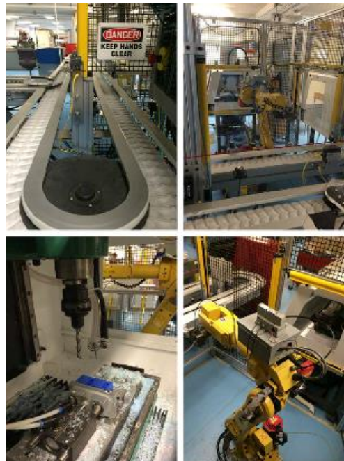
Fig. 2: Various views of the components of SMART. The pictures are of: (a) the main conveyor line (b) Cell 1 (c) CNC and robot from Cell 1 (d) robot from Cell 2
