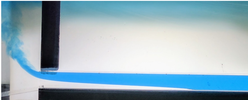
FIGURE 4. A closeup image of an intruding salt wedge during an experiment. Here, freshwater (dyed blue) is observed exiting the channel as a salt wedge intrudes the lower portion of the channel. The freshwater water plume and the diluted mixed layer are visible in the left and upper sections of the image respectively.
