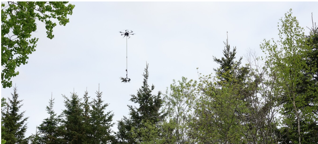
Fig. 1. UAV, equipped with the DeLeaves tool, after collecting a red spruce ( Picea rubens ) sample in Quebec.
