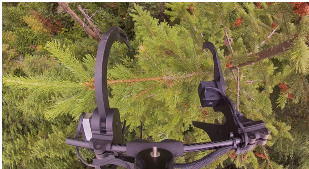
Fig. 12. View from DeLeaves's camera before collecting a branch from a 40 meter Douglas Fir.
