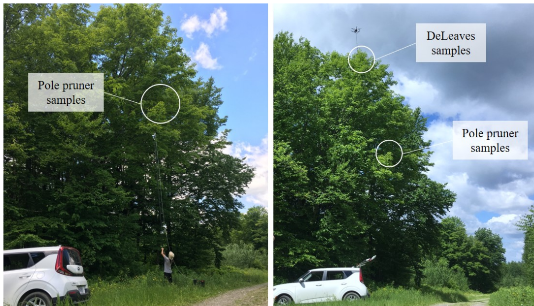
Fig. 11. Comparison of representative sampling locations used with CABO on sugar maple stands in Quebec. Left: pole pruner. Right: DeLeaves tool.
