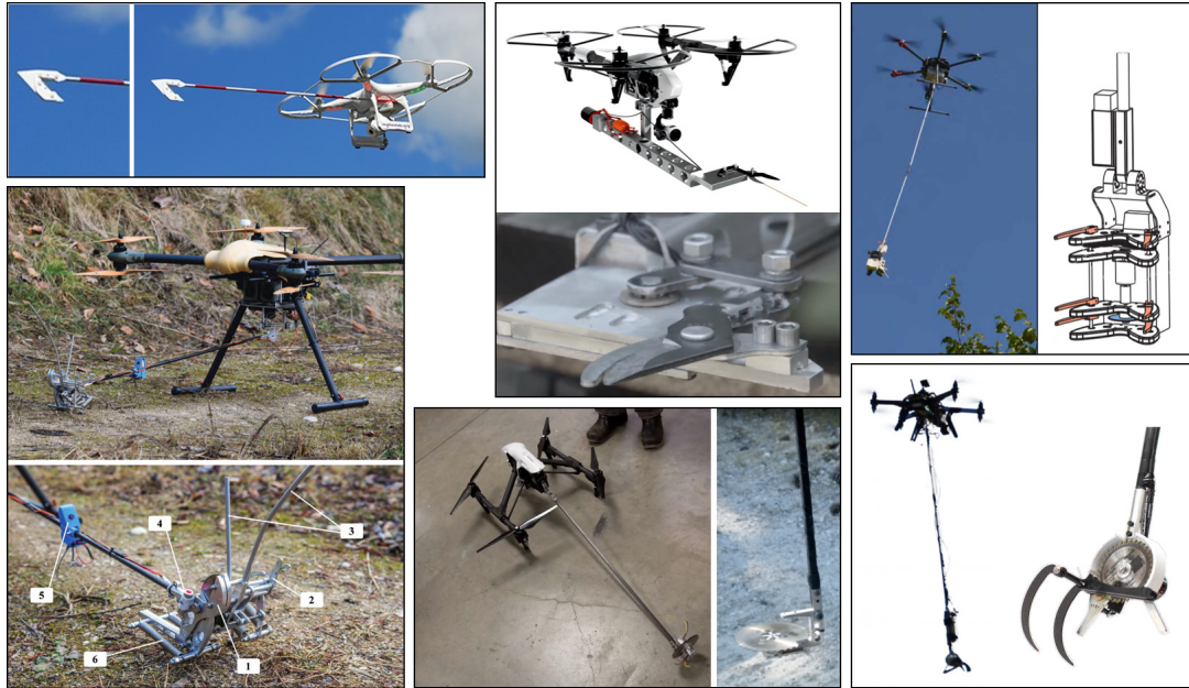
Fig. 3. Tree sampling UAVs from around the world. From left to right, top to bottom: UC Berkeley ( UC Berkeley Forest Pathology and Mycology Lab , 2015), Arborist II from Jamie Hyneman ( Hyneman , 2017), FTTS from ETH Zurich ( Käsliin et al. , 2018), Lucanus from Slovenian Forestry Institute ( Finžgar et al. , 2016), Arborist I from Jamie Hyneman ( Hyneman , 2015), UC Santa Barbara ( Bailey et al. , 2018).
