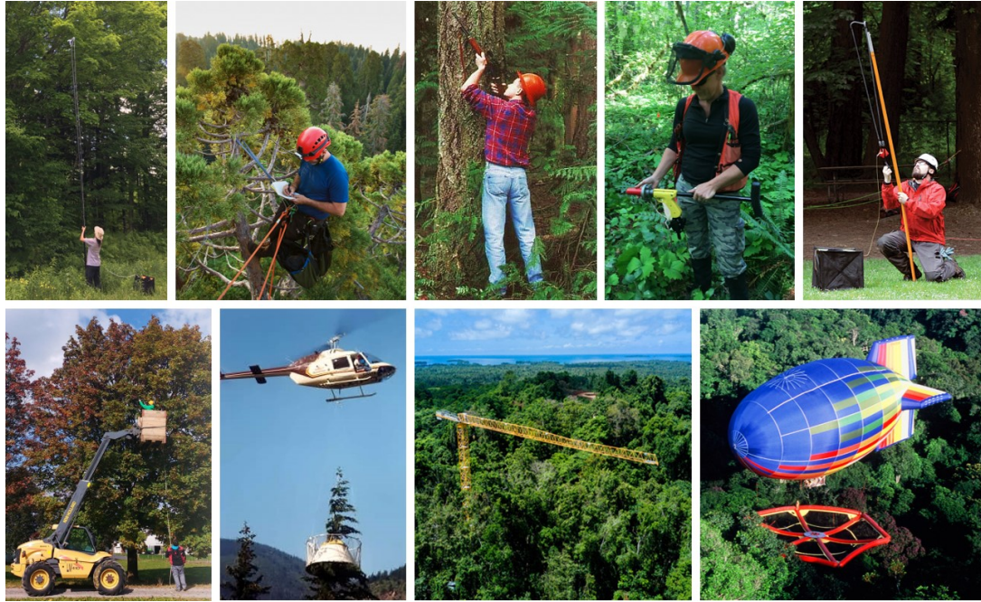
Fig. 2. Tree sampling techniques. Top row, from left to right: pole pruner, climber (Walker, 2016), shotgun (Portlock et al. , 1996), line launcher, slingshot (WesSpur, 2019). Bottom row: hydraulic lift (Käslin et al. , 2018), helicopter (Portlock et al. , 1996), canopy crane (Canopy Crane Papua New Guinea, 2019), canopy raft (Reforest'Action, 2017).
