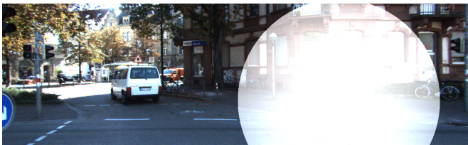
Fig. 2. An example of a compromised camera image that contains a round Gaussian facula.
