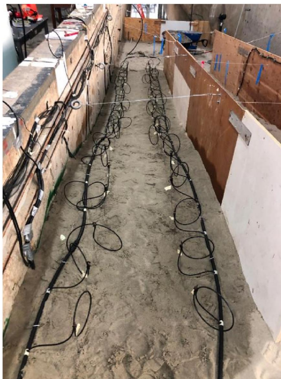
Figure 1. Surface spraying treatment setup.
