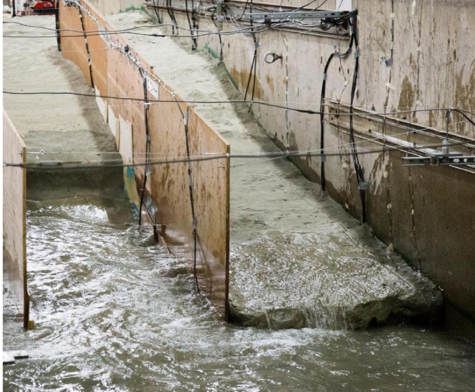
Figure 3. Bio-cemented dune during testing (right) adjacent to the untreated buffer zone (left).
