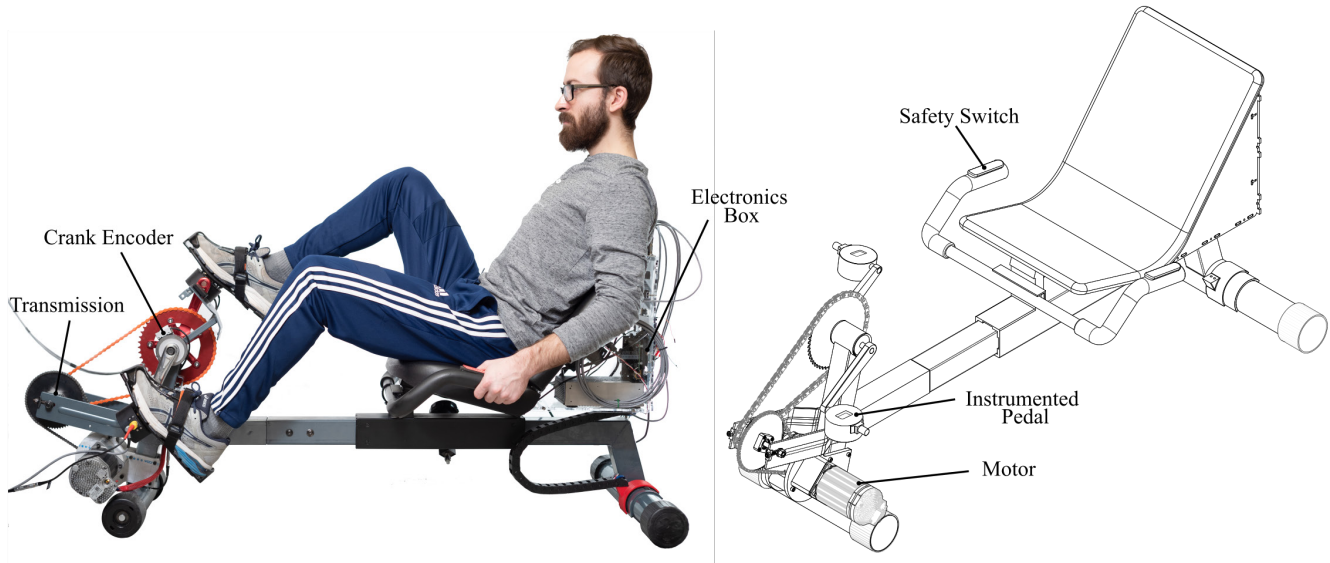
Figure 1 - NOTTABIKE is a one degree-of-freedom robot used to study human motor control and to deliver rehabilitation in the lower-limb. Measurements of subject endpoint kinematics and kinetics are used by a computer controller to create virtual haptic environments.
