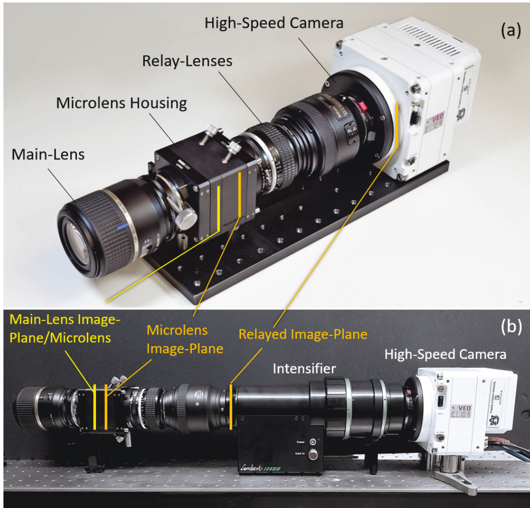
Figure 2. (a) The high-speed relayed-plenoptic camera system with (b) its intensified counterpart.
