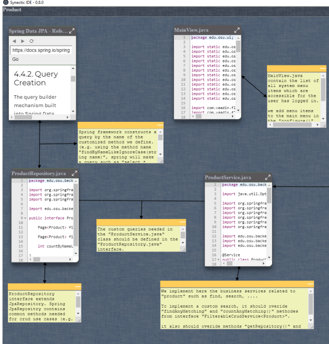
Fig. 1: Synectic provides a canvas-based environment containing spatially arranged cards of relevant information (code, webpages, etc.), along with annotations that link information to individual cards and between related cards. This example groups cards and annotations related to implementing CRUD operations on the product page in Vaadin Bakery App (task T4).
