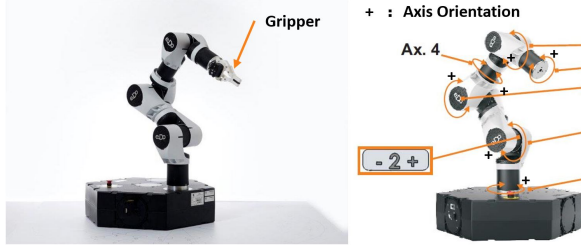
FIGURE 11: THE E.DO ROBOTIC ARM AND POSITIVE ORIENTATIONS OF SIX JOINTS.
