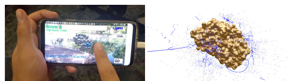
Figure 1: Left: User playing our mobile molecular docking game, DockAnywhere , on an Android phone. Biomolecules displayed are a receptor protein and a ligand. Players move the ligand to find its bound position on the receptor. Right: Ligand position data generated by all players are combined and plotted around the protein receptor. This data is used to find low energy docking pathways.
