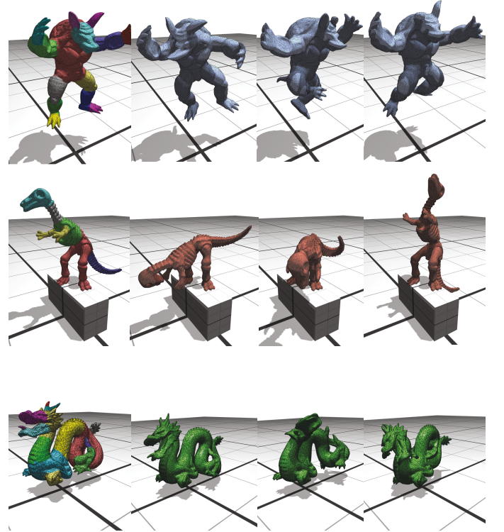
Figure 16: Substructuring allows us to re-use the training data of a regular shape to handle complex deformable bodies. The Armadillo, dinosaur and dragon models use the StVK, co-rotation and Neo-Hookean materials respectively. They use the networks trained with the rectangular beam.
